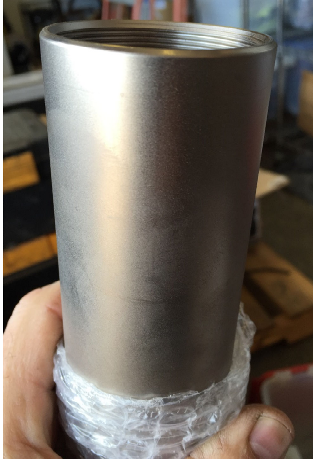
Holmatro Tool Piston Believe this one was large diameter piston for 3350 telescopic ram (also 4350)...
